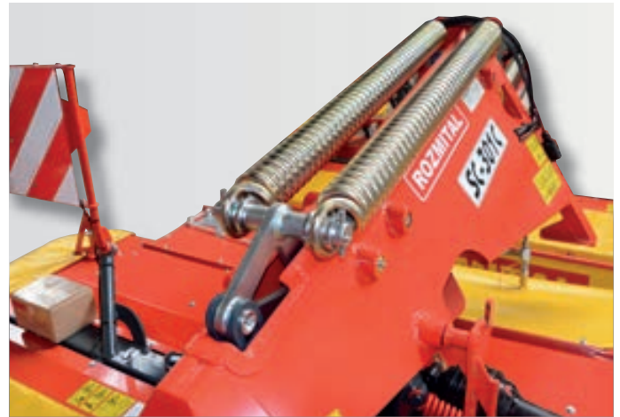
Cutterbar flotation by using springs.
