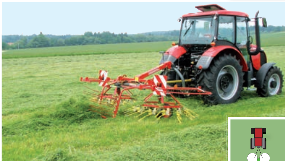
Raking - rod swath guards are in the working position.
