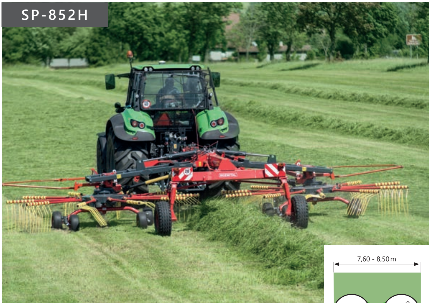
SP-852H mid-row two rotor rake with hydraulically infinitely adjustable working width
