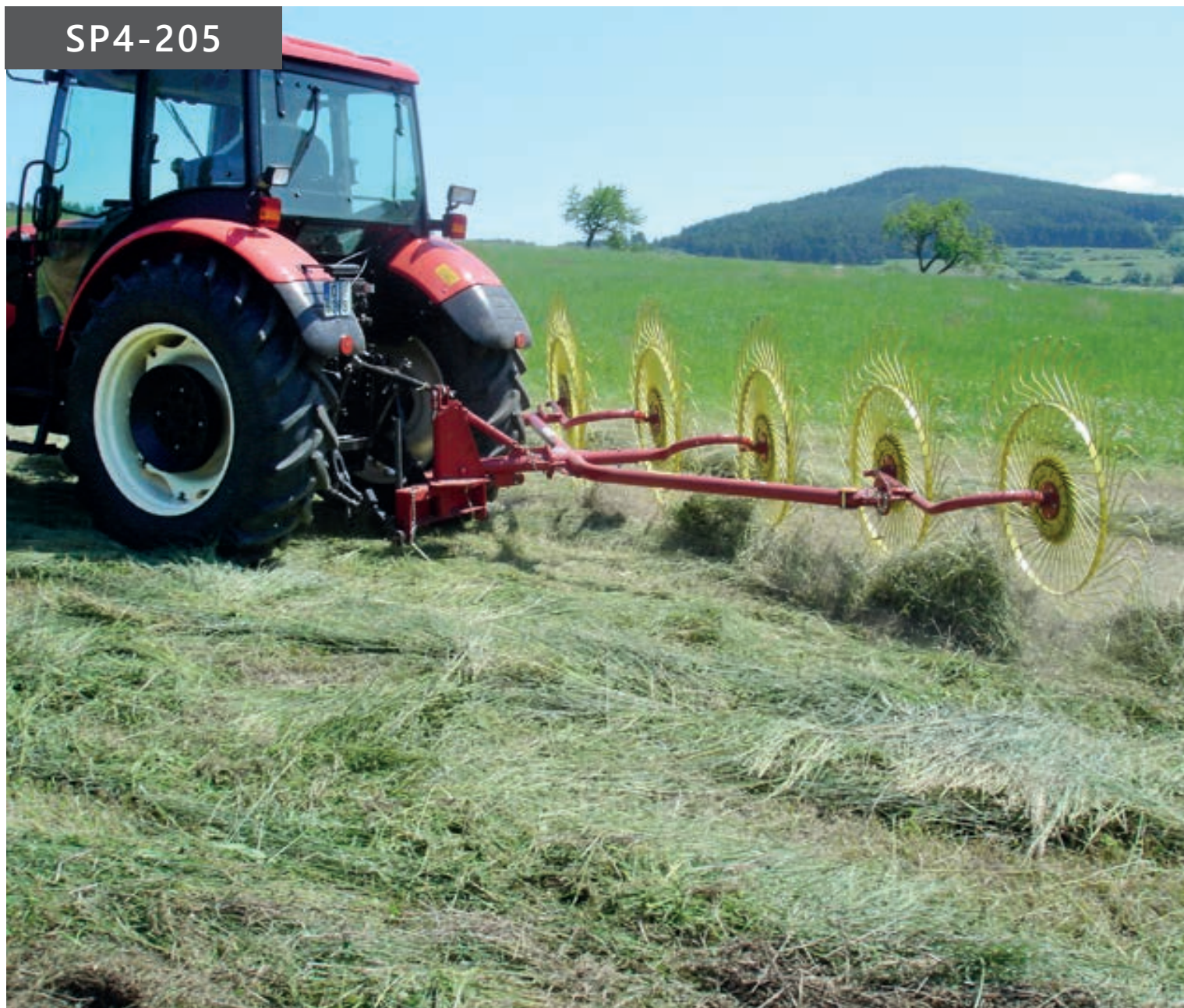
SP4-205 Combined tedder/rake in a single machine
