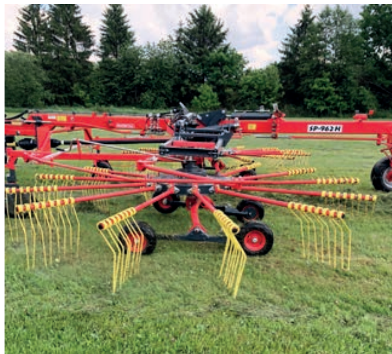
13 arm rotors with a diameter of 4.2 m, 4 double tines per arm
