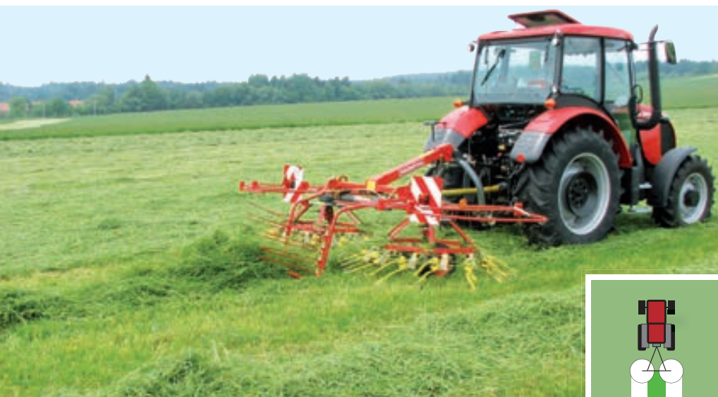
Raking - rod walls are in the working position.
