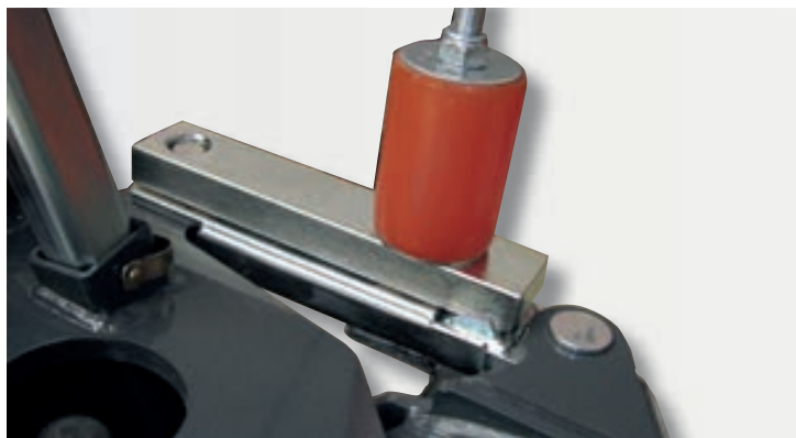
Shock protection system protects the cutterbar against serious damage
