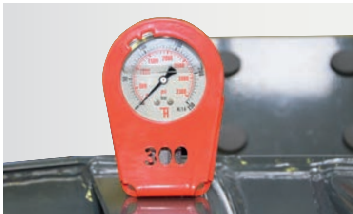
Pressure gauge for easy checking and quick adjustment of the floating position of the side mounted mowers. Basic pressure adjustment is 90-145 bar, depending on the type of machine (1305 - 2103 psi). 90 bar is used as a basic pressure for SD-260 and 145 bar is a basic pressure for SD-300C. The soil conditions (hard, soft, after rain, etc.) must always be taken into account and the pressure adjusted accordingly. Incorrect adjustment of the cutterbar flotation may result in damage to the mower or excessive wear on the skid shoes.
