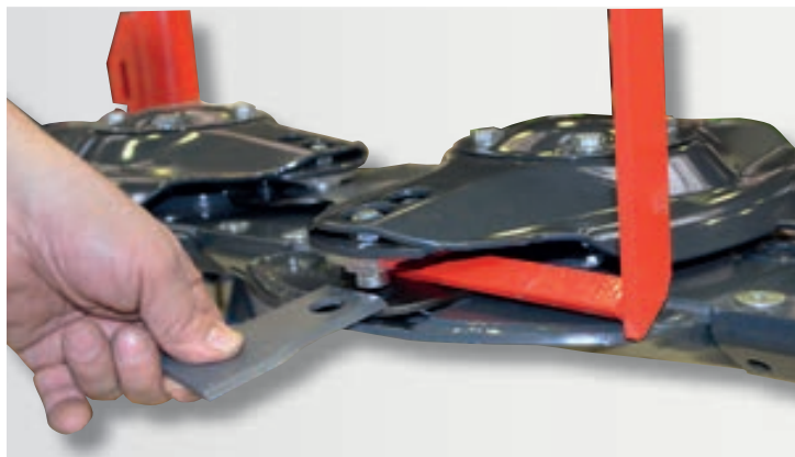
Quick change of the cutting knife using a spring
