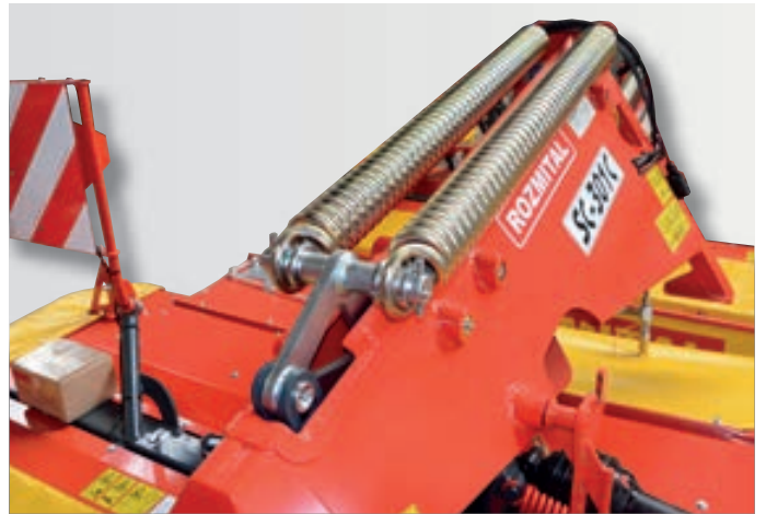
Cutterbar flotation using springs.
