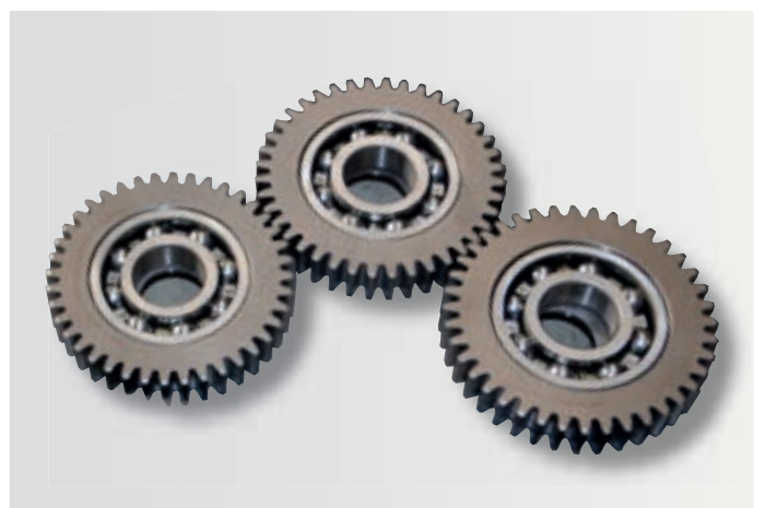
The gears of the cutterbar are forged from high-grade steel with ground tooth edges. The teeth are 22mm wide, on all Rozmital mowers.
