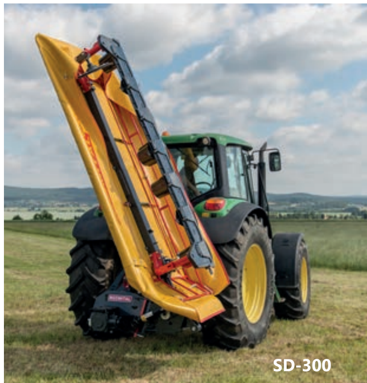
Lift limiter and brake to prevent cutterbar oscillation. If the limiter is in the maximum position, the mower is not properly adjusted. Transport lock for the cutterbar
